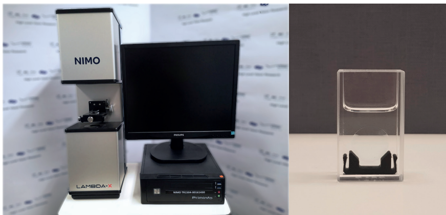
Figure 3: Deflectometer NIMO TR1504 (left) and liquid-filled cuvette with contact lens (right)
