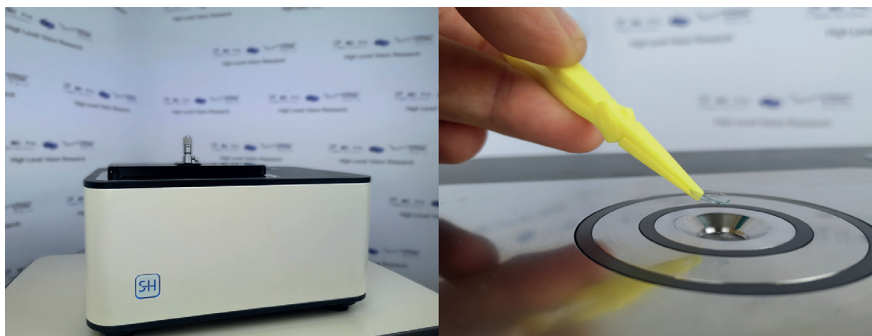
Figure 1: positioning of the contact lens (right) on the VARIREF automatic refractometer (left).
