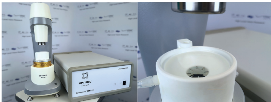
Figure 2: OCT is830 (left) including contact lens wet cell (right)
