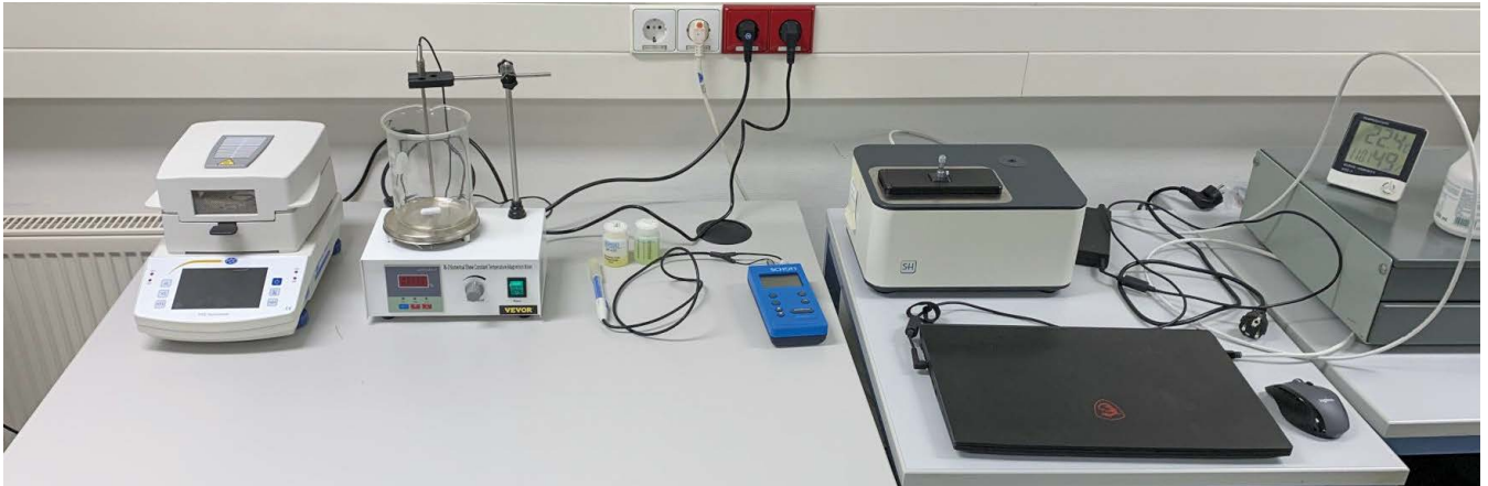
Figure 1: Experimental setup and devices used for the preparation and analysis of the saline solution (from left to right: precision scale, magnetic stirrer, pH meter, refractometer)
